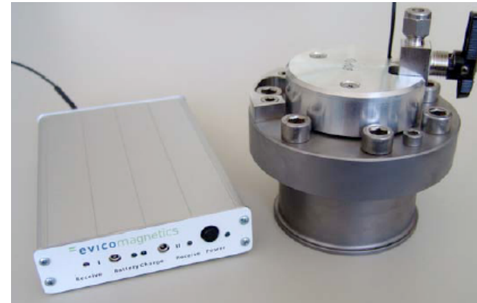
ball milling (Fritsch P6) in Ar, high-pressure vial with pressure/temperature monitoring system (evico magnetics)
